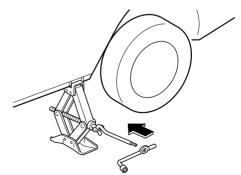
4. Turn the lug wrench clockwise and raise the vehicle high enough so that the spare tire can be installed. Before removing the lug nuts, make sure your Mazda is firmly in position and that it cannot slip or move.
